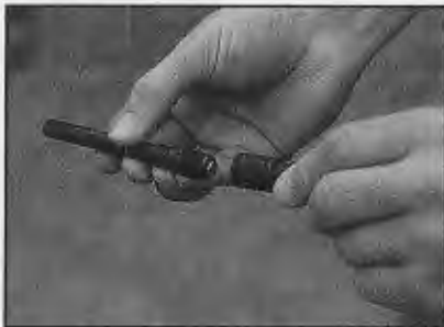
With a round in the chamber, the firing mechanism is screwed on.
